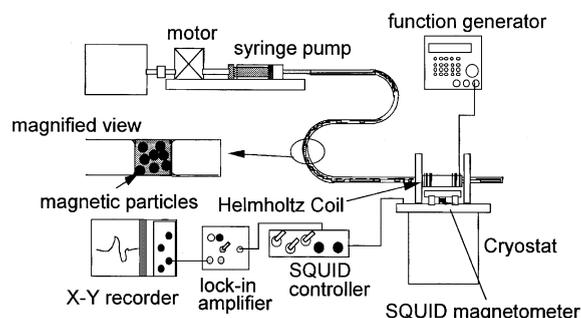
Fig. 2. Schematic diagram of the system for the feasibility test. A pair of coils were mounted just above the SQUID cryostat. External AC magnetic field was applied by the coils. A motor driven syringe pump was employed to push the magnetic particle sample inside a thin tube. The modulated signal associated with the particle motion was demodulated by the lock-in amplifier.
