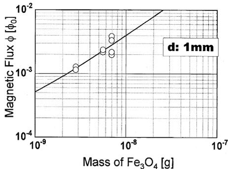
Fig. 6. Magnetic flux vs. mass of iron contained in the sample. Magnetic flux signal was proportional to the weight of the iron in the fluid. Particles of 2.8 ng in weight of iron would be detected with a spacing of 1 mm.
