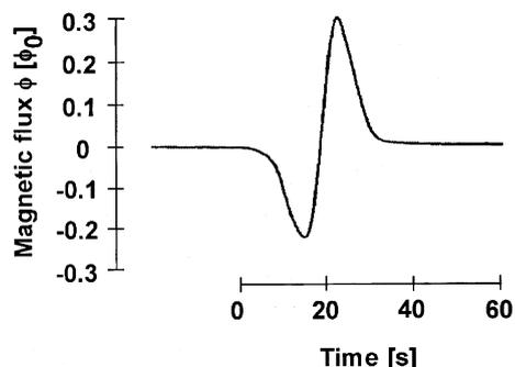
Fig. 3. Typical output signal from the lock-in amplifier. Each positive and negative peak was observed when each edge of the fluid specimen passed over the center of the SQUID.
