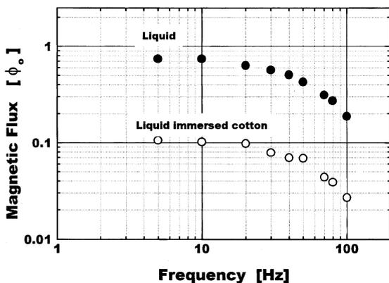
Fig. 4. Frequency dependence of the output signal. The modulation frequency of the Helmholtz coil was changed from 5 to 100 Hz. Closed circles show the results from liquid sample. Open circles show the results from liquid with a piece of cotton.
