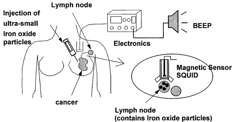
Fig. 1. The system diagram of the sentinel-node biopsy using high- $T_c$  SQUID, which we are proposing. The particles would be injected into the breast; and the high- $T_c$  SQUID is used as a sensing detector for the particles. This method has an advantage of no radiation exposure.
