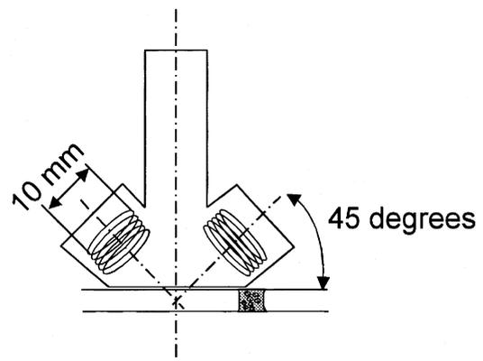
Fig. 5. Schematic drawing of the practical coil design. A pair of 1000 turn wound coils was set with angle of  $90^\circ$ . Tube with a fluid sample was located under the coil and the signal from the sample was measured by the SQUID under the tube.
